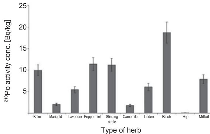
Fig. 1. Measured 210 Po concentration of medicinal herbs (error bars mean the standard deviation from the measurement of 3 parallel samples).
