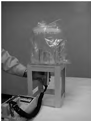
Fig. 2. Assembly for calibration using a reference solution filled in a typical 2L Marinelli beaker.
