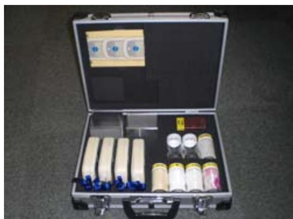
**Fig. 4-1.** Experiment kit to test radiation features using Hakaru-kun.
