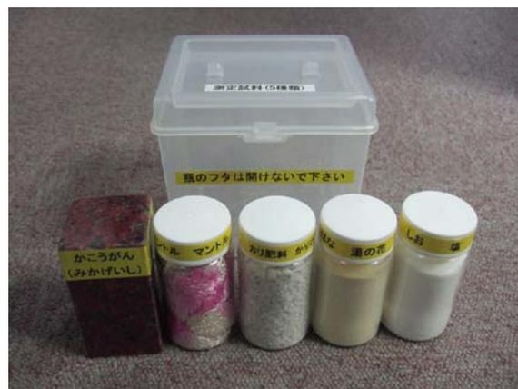
**Fig. 3.** Radioactive sample kit for measurement by Hakaru-kun.
