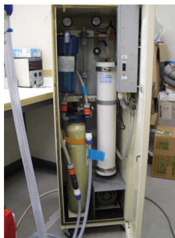
Photo. 4 The industrial RO reverse osmosis membrane.
