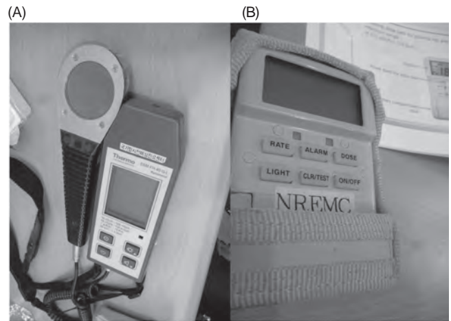
Fig. 2. Survey meter (A) and Personal Dosimeter (B) made in South Korea.
