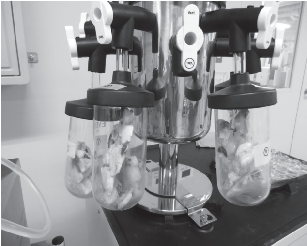
Fig. 3. Multiple drying containers in our tritium measurement pretreatment system.
